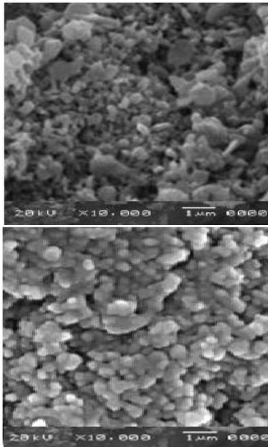
Figure 3. SEM images of (a) PEG:  $\text{CuFe}_2\text{O}_4$  and (b) CTAB:  $\text{CuFe}_2\text{O}_4$  nanoparticles calcined at  $650^\circ\text{C}$
