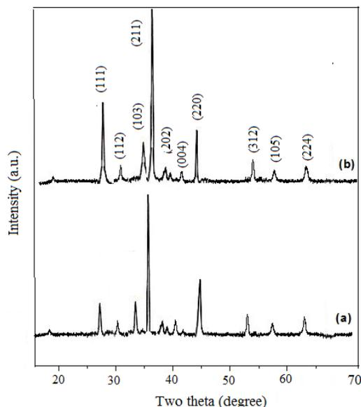
Figure 1. XRD patterns of (a) PEG:  $\text{CuFe}_2\text{O}_4$  and (b) CTAB:  $\text{CuFe}_2\text{O}_4$  nanoparticles calcined at  $650^\circ\text{C}$
