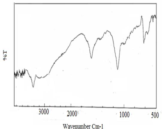
Figure 2. FT-IR spectrum of PEG:  $\text{CuFe}_2\text{O}_4$  nanoparticles calcined at  $650^\circ\text{C}$ .
